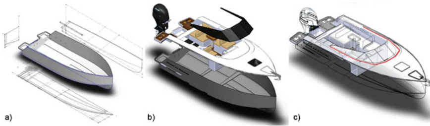
Fig. 4 3D modelling process: a individual modelling of components; b components assembly; c analysis of interferences and clearances of the various components
