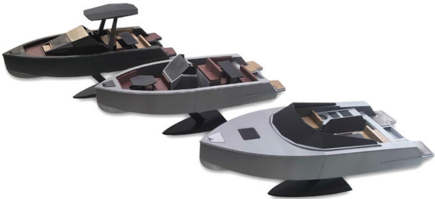
Fig. 19 Prototypes produced by additive manufacturing: Walkaround version, Open version and Classic version (from left to right)
