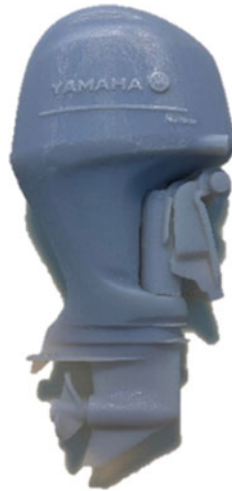
Fig. 18 3D printing of the craft's engine using PolyJet technology
